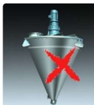
Single cone mixer Volum < 5000L 60% loading rate
