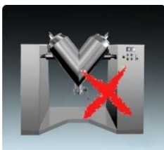
V type mixer Small volume 45% low loading rate
