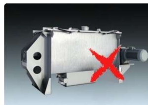
Ribbon mixer Bad mixing uniformity 65% loading rate
